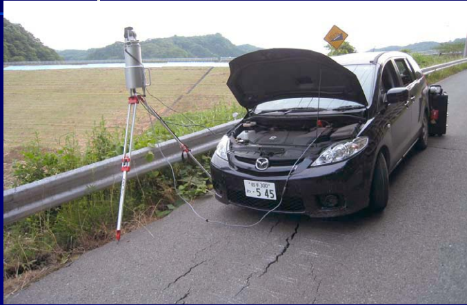
LIDAR scans of susceptible dams (from GEER, Japan 2008 EQ)
