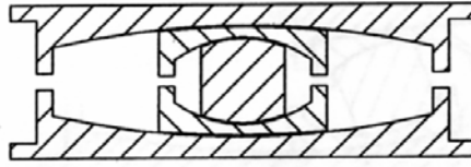
Figure 6: Section through Triple Concave FP bearing
