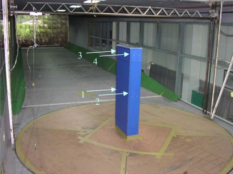
Fig. 16 : 1/160 Scaled Building Model Subject to the Actuating Force under Smooth Flow
