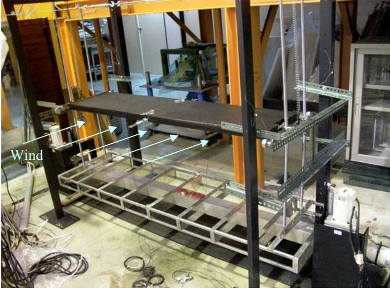
Fig. 17 : Bridge Section Model Excited by a two-axis Actuating Device
