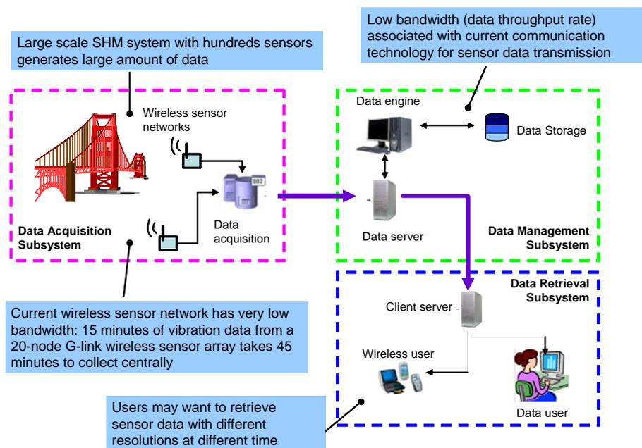
Figure 1. Schematic of a modern structural health monitoring system with wireless communication
