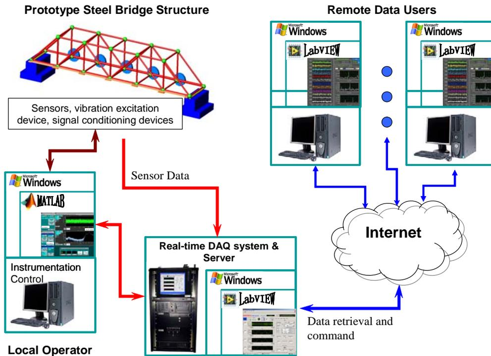
Figure 2. Schematics of the prototype integrated SHM system at Lehigh University
