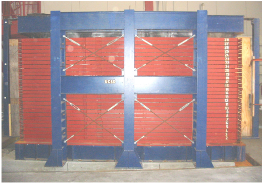
Figure 3. The UCSD medium size laminar box (Jakrapiyanun, 2002).
