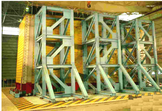
Figure 1. The NIED large size laminar box (Kagawa et al., 2004).
