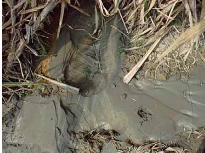
Figure 2. Sand boils in a rice field at Chingliao during the Chiayi earthquake
