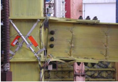
Figure 6. RFP buckling (Specimen RFP-1).
