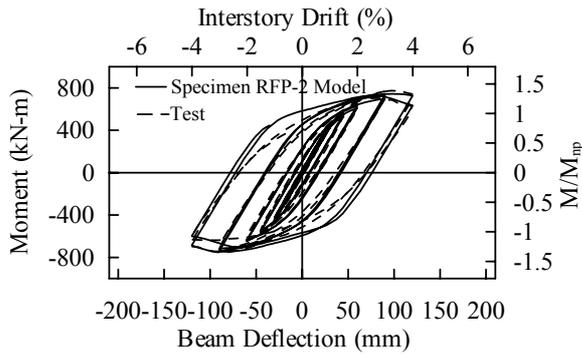
(a) Specimen RFP-2 model versus test result
