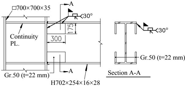
Figure 3. Specimen RMC-2 connection details.
