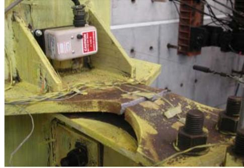
Figure 7. RFP fracture (Specimen RFP-2).
