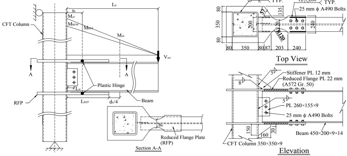
Figure 1. Moment distribution along beam length. Figure 2. Specimen RFP-2 connection details.
