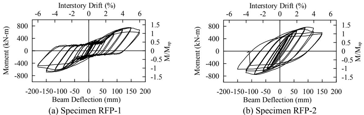
Figure 5. Moment versus beam deflection relationship (weakened moment connections).
