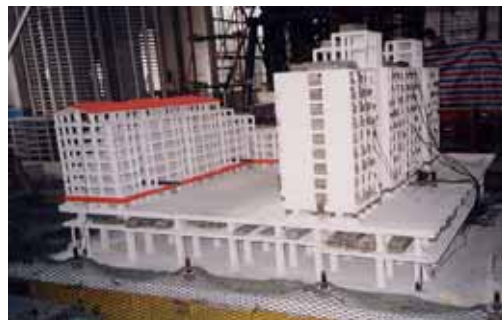
Figure 11: Shaking table tests for structural model of IHBSH
