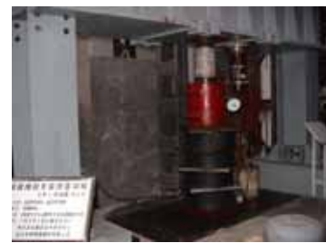
Figure 1: Design of rubber bearing Figure 2: Comp.--shear test for bearing Figure 3: Tests of Creep
