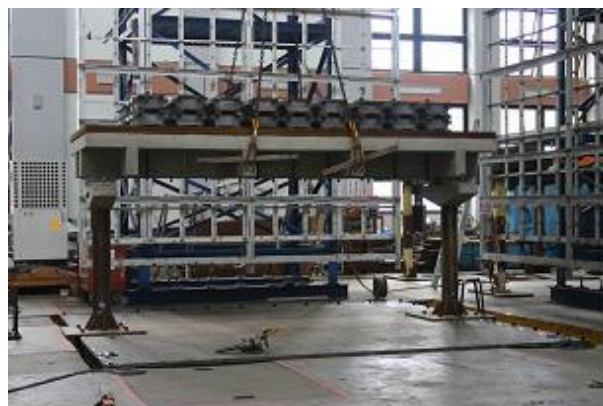
Figure 3 The 1/7.5 isolated bridge model.
